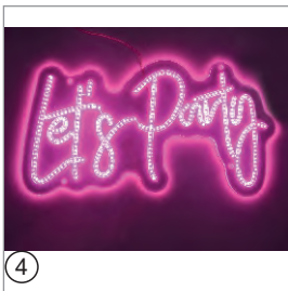
4. Give power to LED strip to test if all LED strip in good quality.
