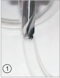
1. Carve a groove with a milling cutter.
