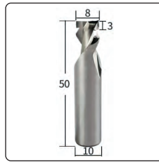
Milling Cutter It is used on CNC machine, to carve groove for neon signs, strip width 6 mm, base plate thickness \geq 6 mm, cutting depth 4.2 mm
